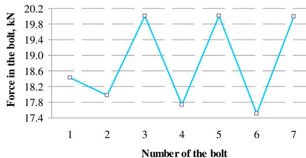
Fig. 5. Preload values at the end of the assembly process
