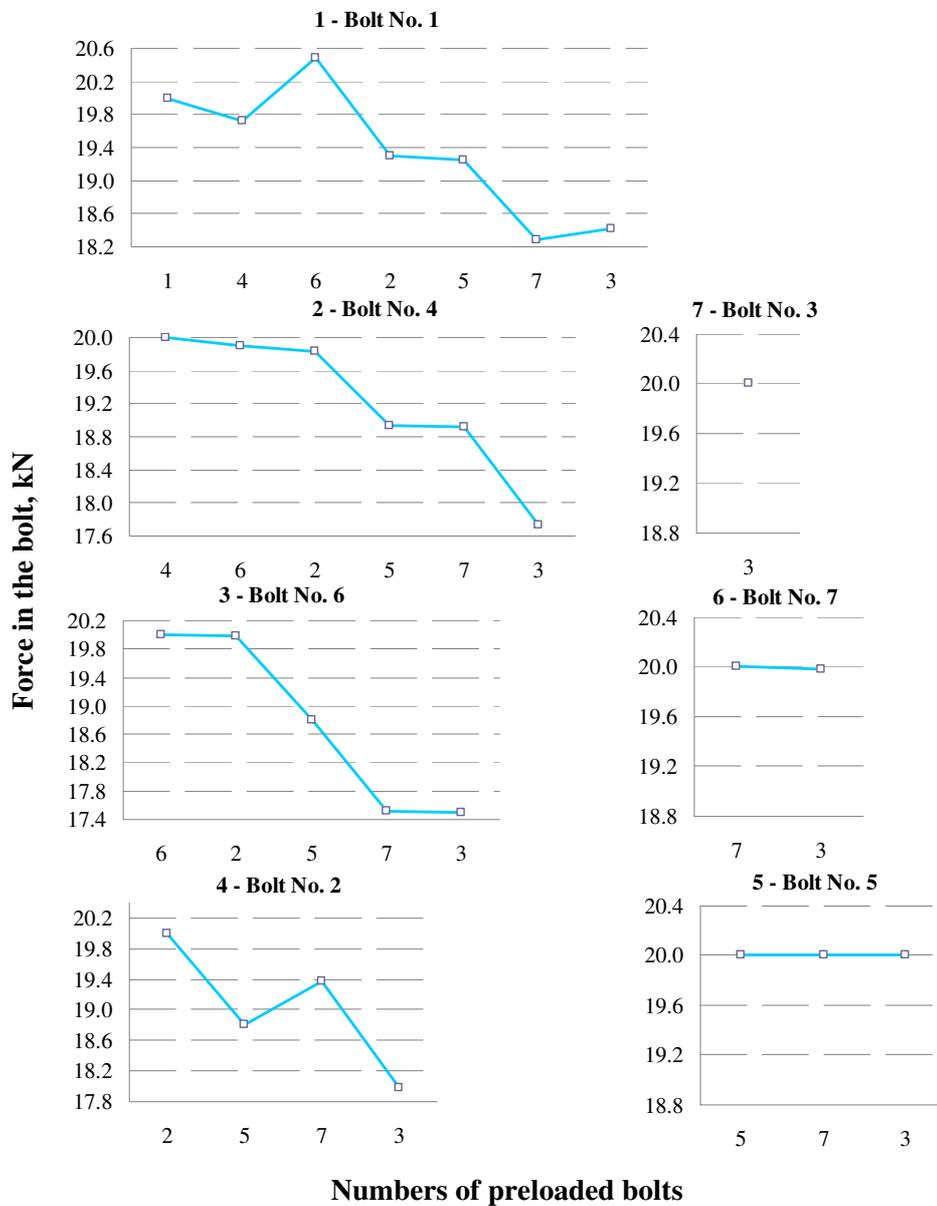
Fig. 4. Preload values during the assembly process
