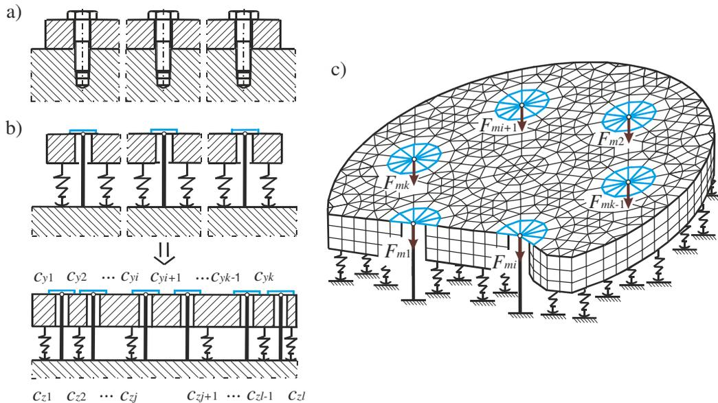
Fig. 1. **Multi-bolted connection:** a – scheme; b – description of spring properties; c – FEM-model with spider bolt models
