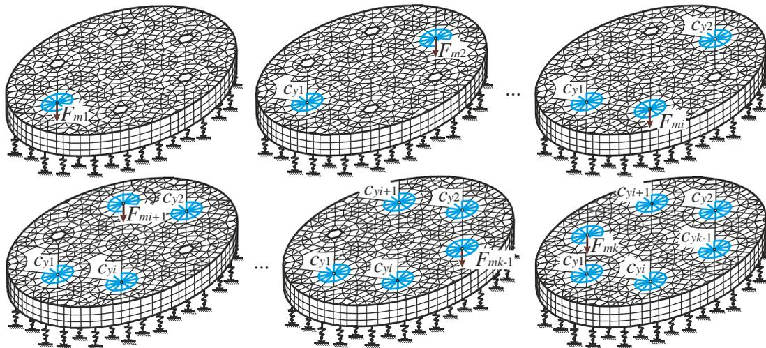
Fig. 2. Preloading process of the multi-bolted connection
