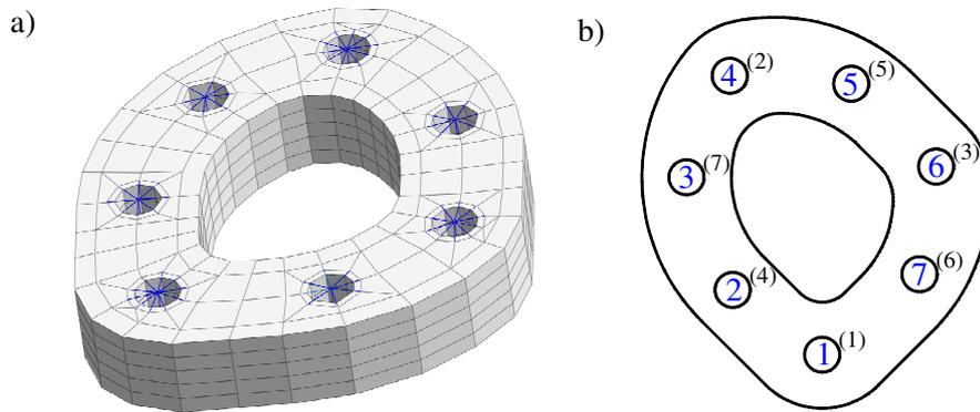
Fig. 3. Considered multi-bolted connection: a – simplified FEM-model; b – contact surface
