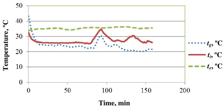
Fig.1. Temperature in combine harvester operator driving cabin
