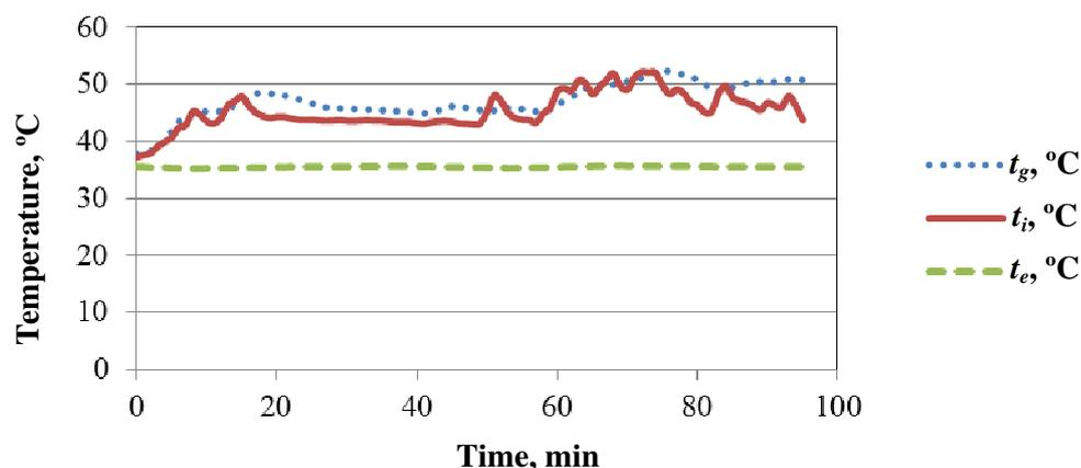
Fig. 2. Temperature in tractor operator driving cabin
