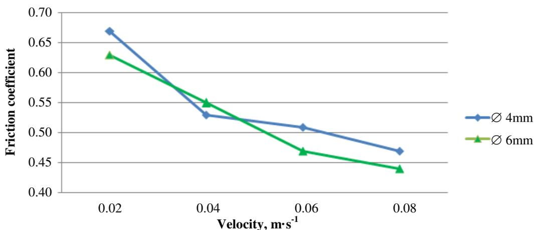
Fig. 2. Granule kinetic friction coefficient dependency on sliding velocity on plastic surface
