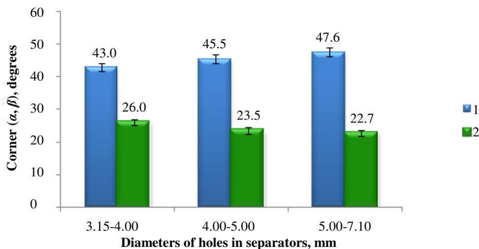
Fig. 3. Natural slope and inrush failure angle dependency on granule diameter:
