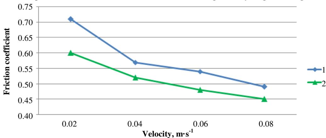
Fig. 1. Granule kinetic friction coefficient dependency on sliding velocity on metal surface:
