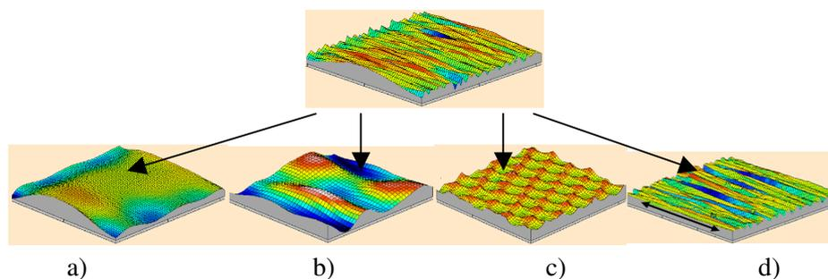
Fig. 2. Surface texture: a – shape, b – waviness, c - roughness, d – direction of roughness [3]
