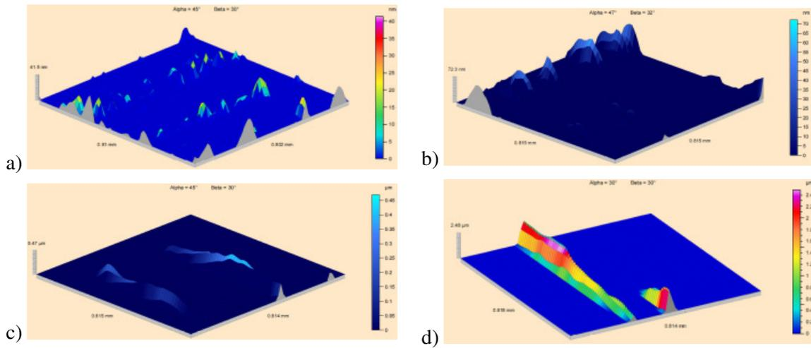
Fig. 5. Volume of surfaces' No.1 (a), No.3 (b), No.6 (c), No.8 (d) separated material during running-in stage
