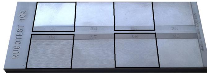
Fig. 1. Flat grinded sample Rugotest 104
