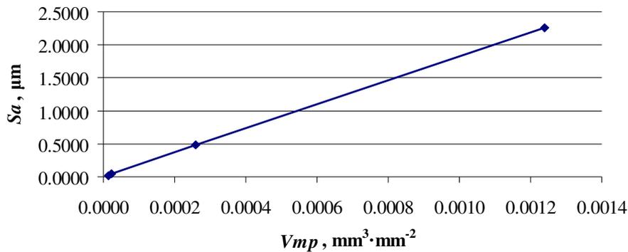
Fig. 6. Dependence between parameters  $S_a$  and  $V_{mp}$
