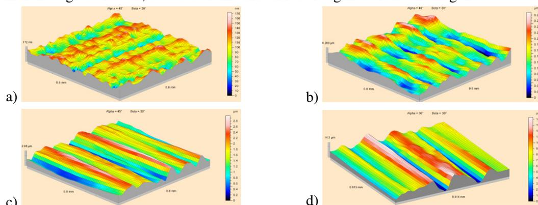
Fig. 3. Topography of roughness of surfaces No.1 (a), No.3 (b), No.6 (c), No.8 (d)
