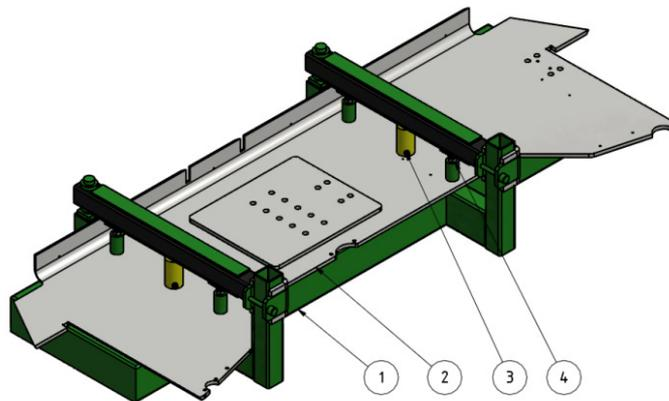
Fig. 5. Overview of breaking jig: 1 – breaking jig; 2 – plane; 3 – cylinder; 4 – tensioner
