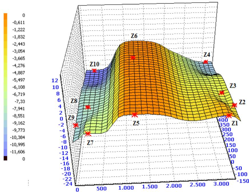
Fig. 4. Bending strain of plate after welding
