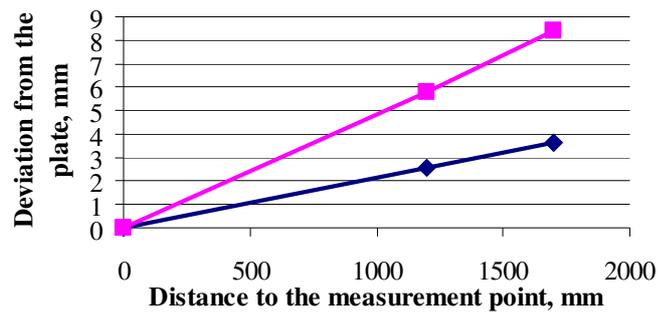
Fig. 7. **Bending deformations of plates after welding:** without using of indirect bends (upper curve); with using of indirect bends (bottom curve)
