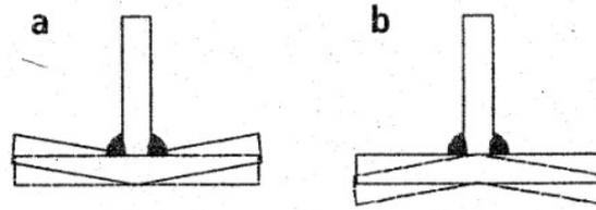
Fig. 1. **Scheme of formation of deformations:** a – welding without using of indirect bend;
