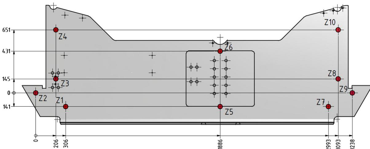
Fig. 2. **Part dimensions in plane and measurement scheme**
