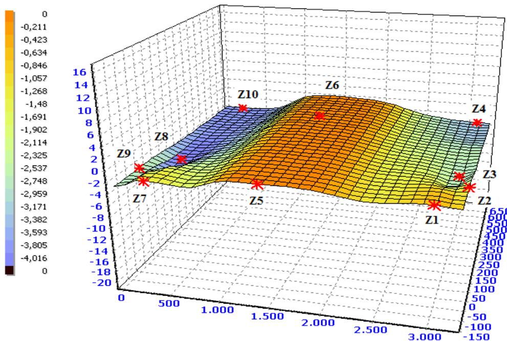
Fig. 6. Deformations of plate after welding, by using of breaking jig
