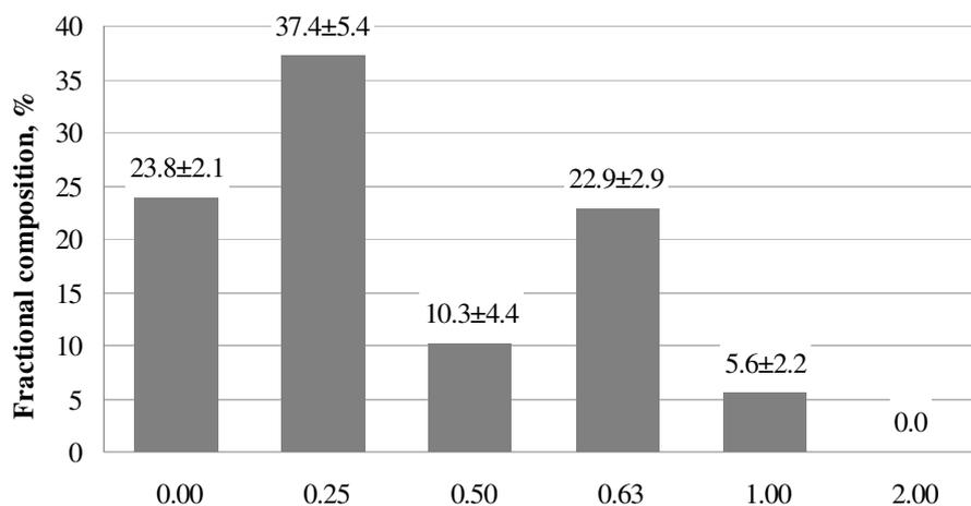
Fig. 3. Fraction composition of oak bark and leaves mixture mill (diameter of holes in mm)
