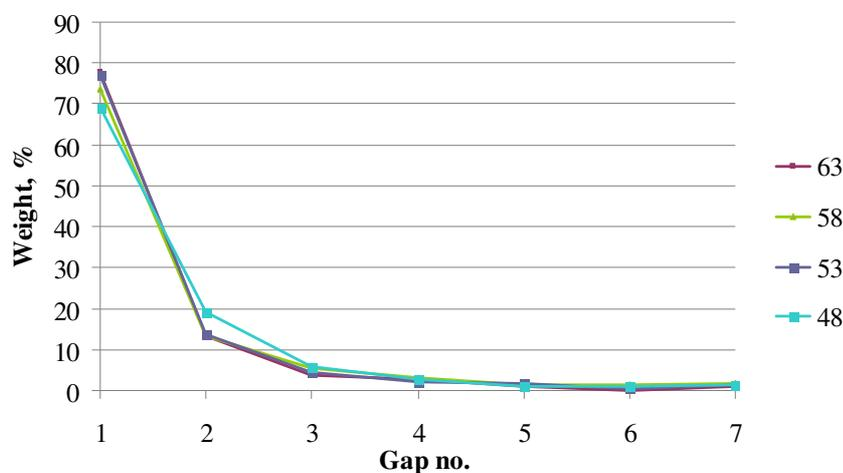
Fig. 3. Weight percentage of fall through in the gaps between the rollers
