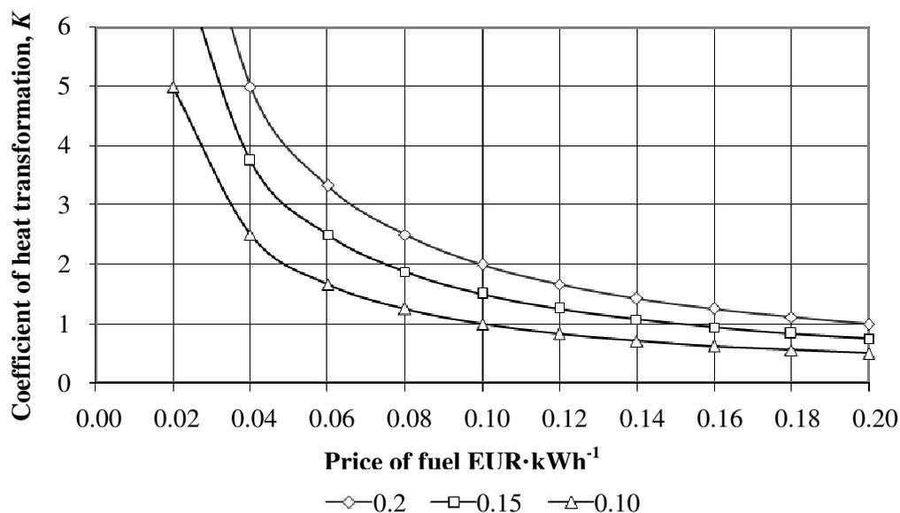
Fig. 2. Coefficient of heat transformation at which the use of a heat pump starts to be economic at the price of electric energy 0.1; 0.15 and 0.20 EUR·kWh<sup>-1</sup>
