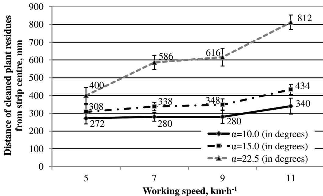
Fig. 5. Working speed and row cleaner attack angle influence on the cleaned off crop residues distance from the centre of the strip, where  $L = 135$  mm
