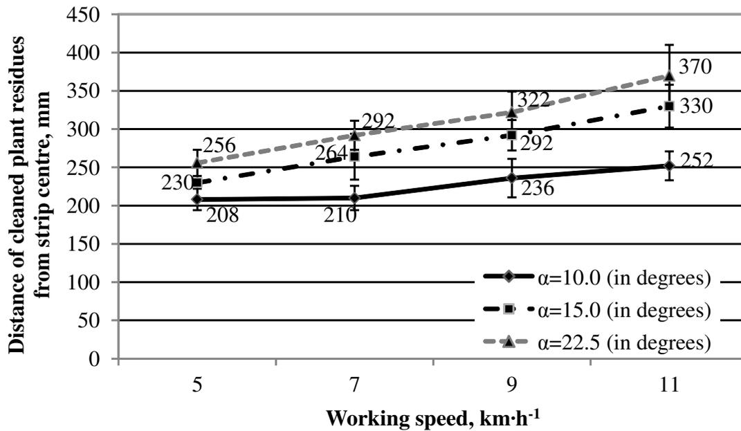
Fig. 3. Working speed and row cleaner attack angle influence on the cleaned off crop residues distance from the centre of the strip, where  $L = 105$  mm
