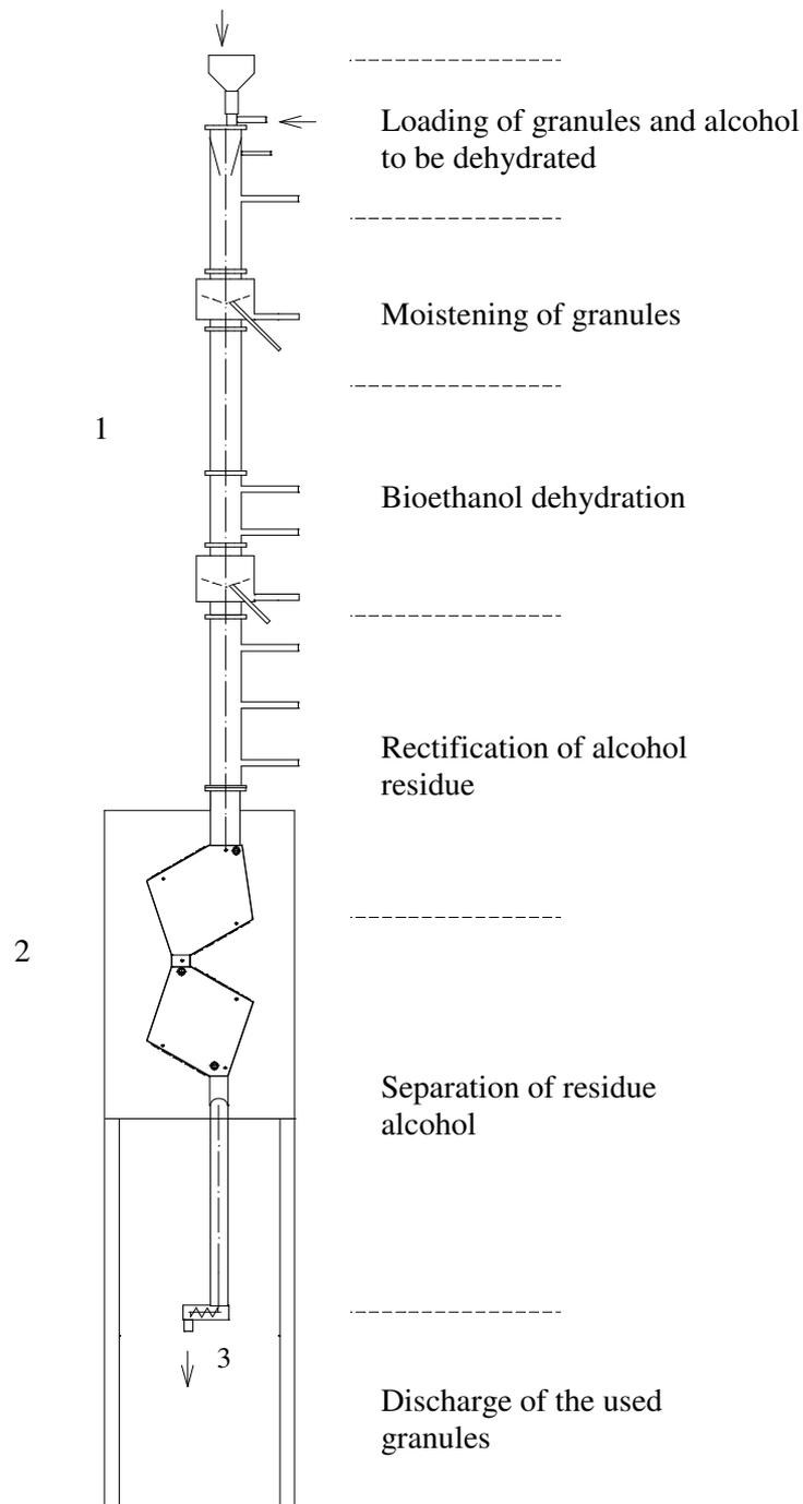
Fig. 1. A principal scheme of the experimental equipment
