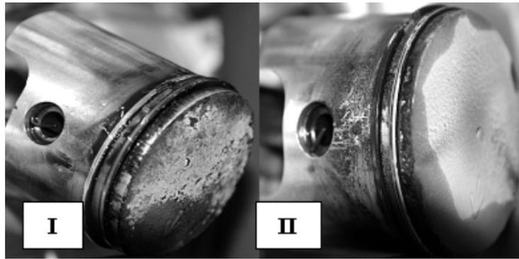
Fig. 4. Comparison of residues on the piston with the tested generators I and II
