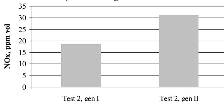
Fig. 9. Comparison of the amounts of NO<sub>x</sub> contained in exhaust gases in Test 2
