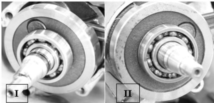
Fig. 5. Comparison of corrosion with the tested generators I and II
