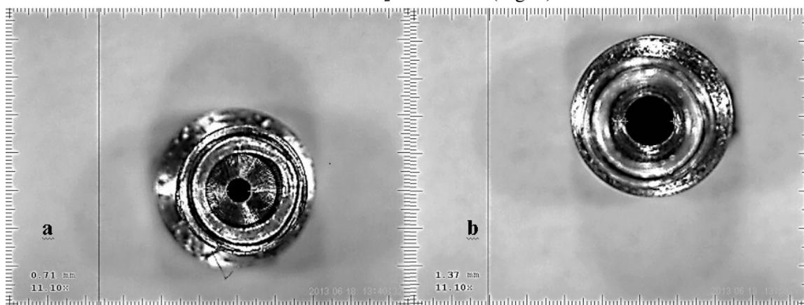
Fig. 2. Non-modified nozzle port (a) and modified nozzle port (b) of the generator II
