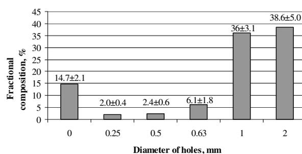
Fig. 6. Fraction composition of common mugwort mill
