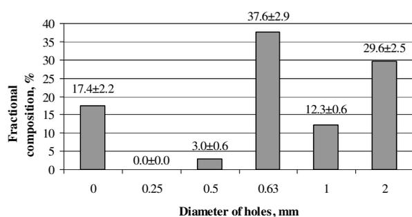
Fig. 5. Fraction composition of cup plant mill
