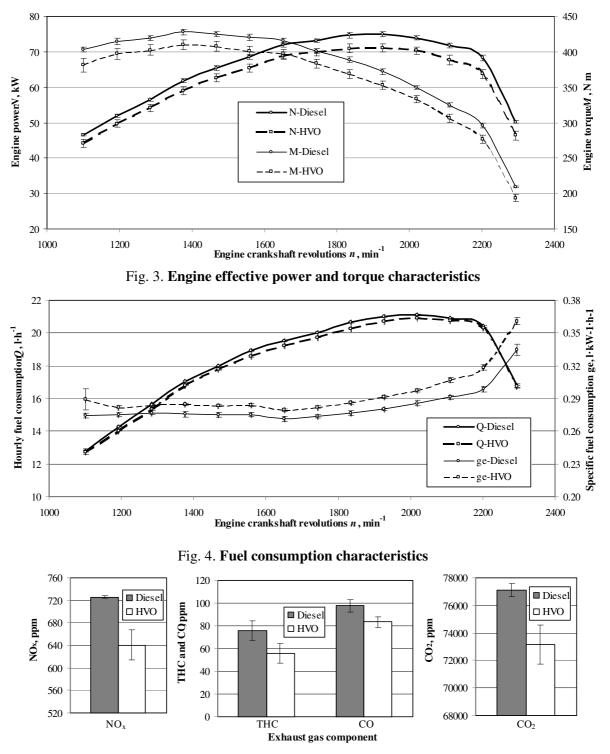
Fig. 5. Content of NO<sub>x</sub>, THC, CO and CO<sub>2</sub> in exhaust gases
