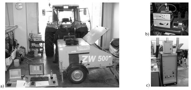
Fig. 1. Test object and measuring equipment: a – CLAAS ARES 557ATX and MAHA ZW-500; b – AVL KMA MOBILE; c – AVL SESAM FTIR
