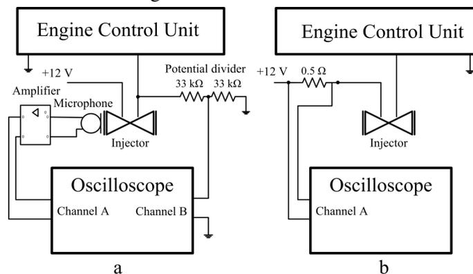
Fig. 1. Principal connections of the test setup:
