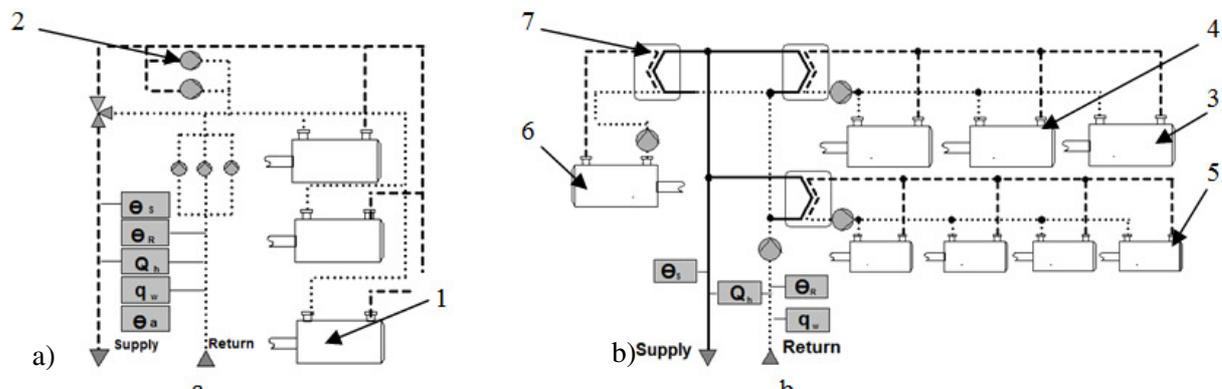
Fig. 1. **Block diagram of the city municipal DH plant setup:** a – Cesis city; b – Jelgava city;
