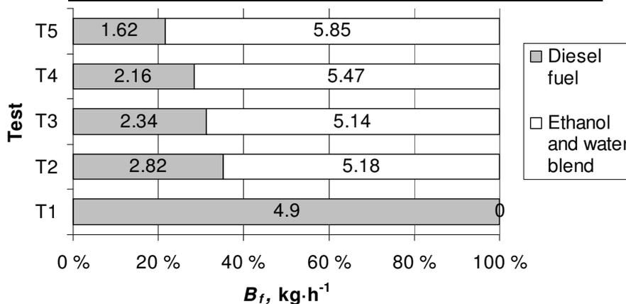
**Fig. 2. Absolute fuel quantities and relative proportion used in testing when comparing diesel fuel and ethanol**
