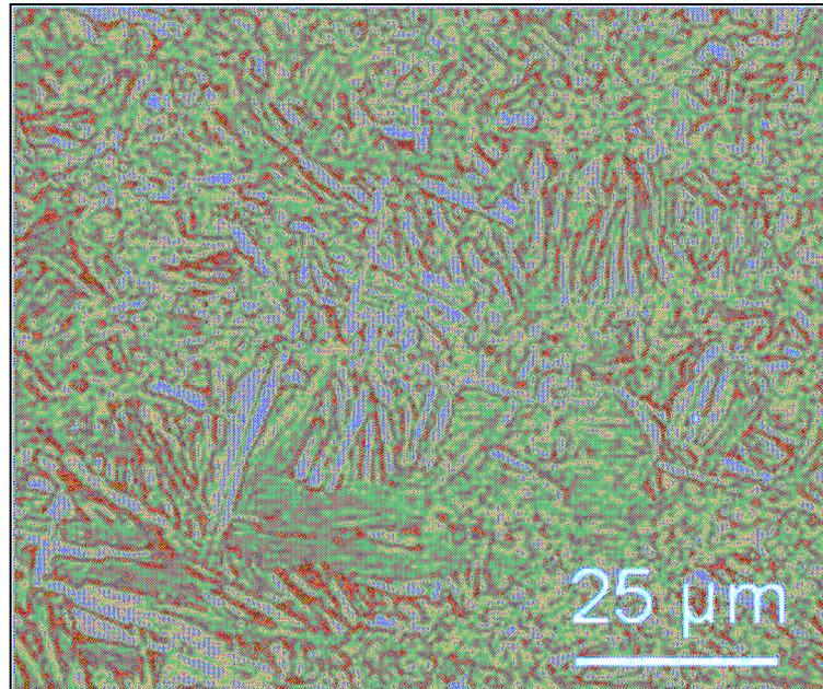
Fig.1 Initial structure of Ti-alloy, without corrosion load
