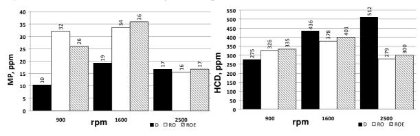
Fig. 3. MP and HCD measurement results: D - diesel fuel, RO - pure oil, ROE - enriched oil
