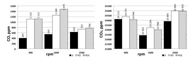
Fig. 2. CO and CO<sub>2</sub> measurement results: D – diesel fuel, RO – rapeseed oil, ROE – enriched oil
