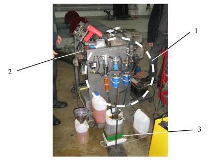
Fig. 1. **Engine test bench:** 1 – *Elsbett* two-tank system; 2 – diesel engine; 3 – weighing system
