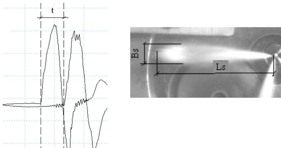
Fig. 1. Principle of sound velocity and fuel spray parameter measurement
