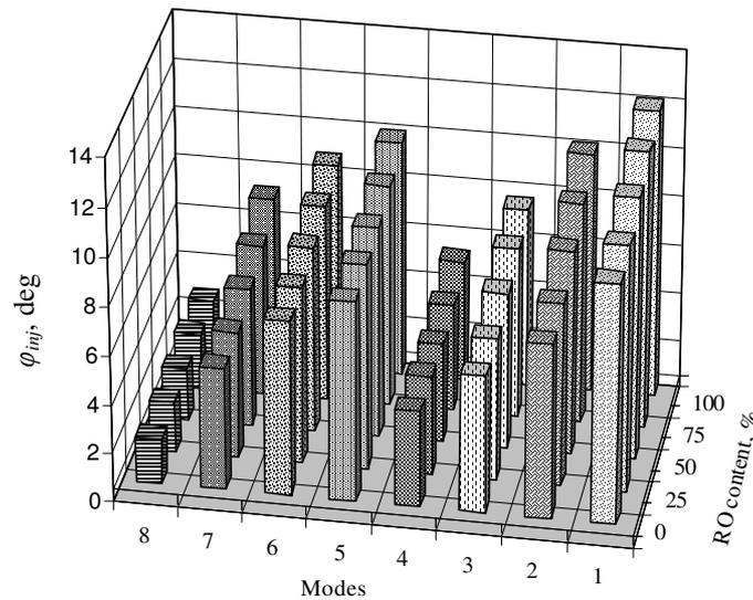
**Fig. 3. Fuel injection duration in degrees of crankshaft angle as a function of performance mode and rapeseed oil content in fuel**
