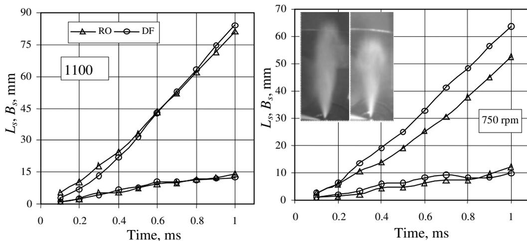
**Fig.4. Fuel sprays tip penetration  $L_s$  and spray width  $B_s$  as a function of time**
