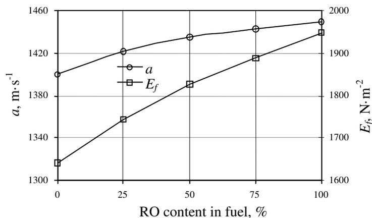
Fig. 2. Sound velocity in fuel ( $a$ ) and fuel bulk modulus ( $E_F$ ) as a function of rapeseed oil content in fuel
