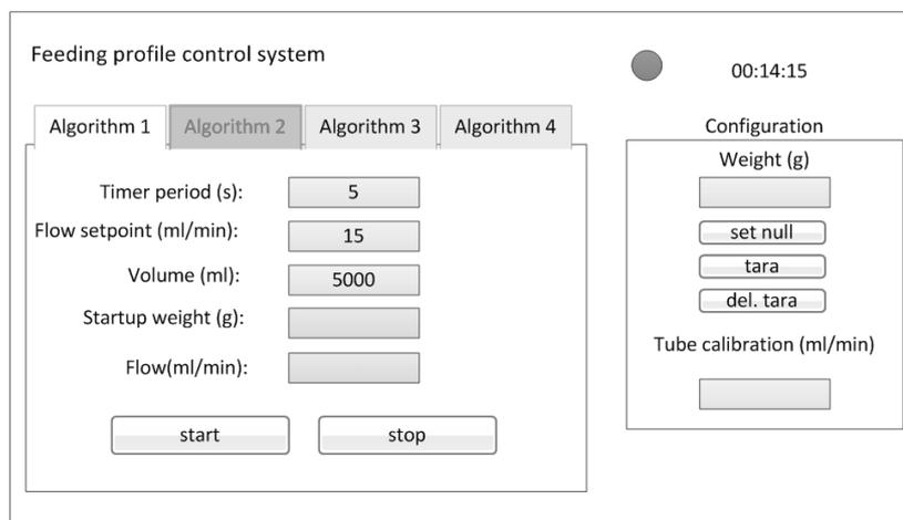
Fig. 6. User interface on HMI
