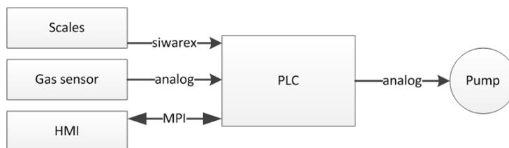
Fig. 3. Communication scheme in system
