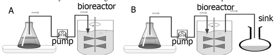
Fig. 1. Schemes of fermentation processes: A – fed-batch, B – continuous
