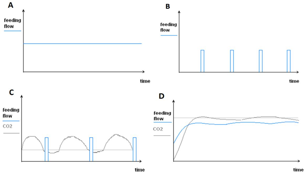
Fig. 5. Time diagrams of feeding processes
