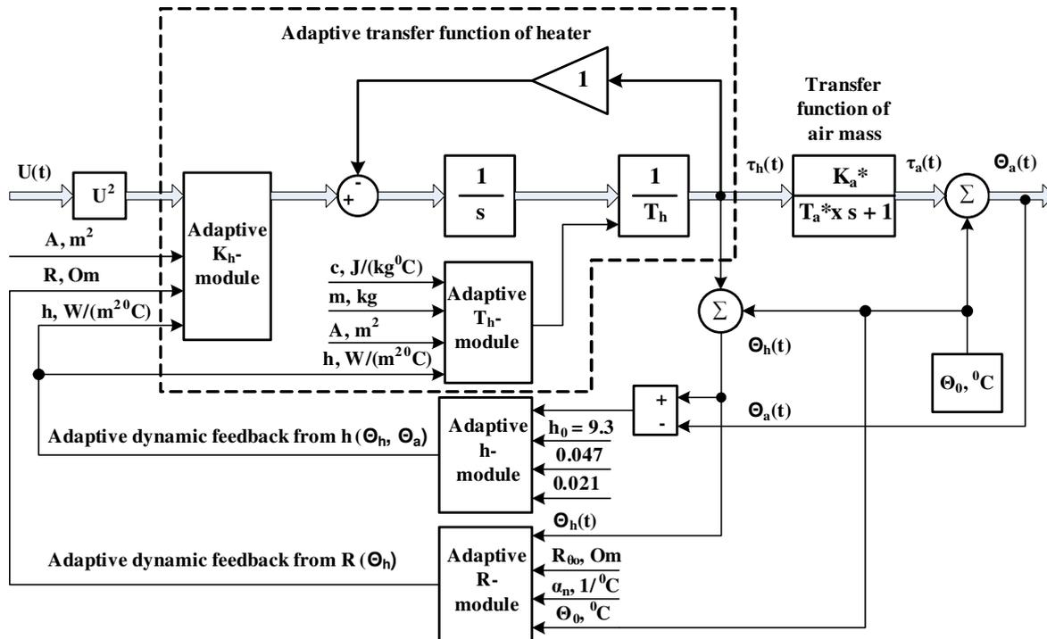
Fig. 1. Adaptive self - tuning up model of electrical heater with adaptive dynamic feedbacks from temperature dependent heat transfer coefficient  $h(\Theta_h, \Theta_a)$  and from heater resistance  $R(\Theta_h)$
