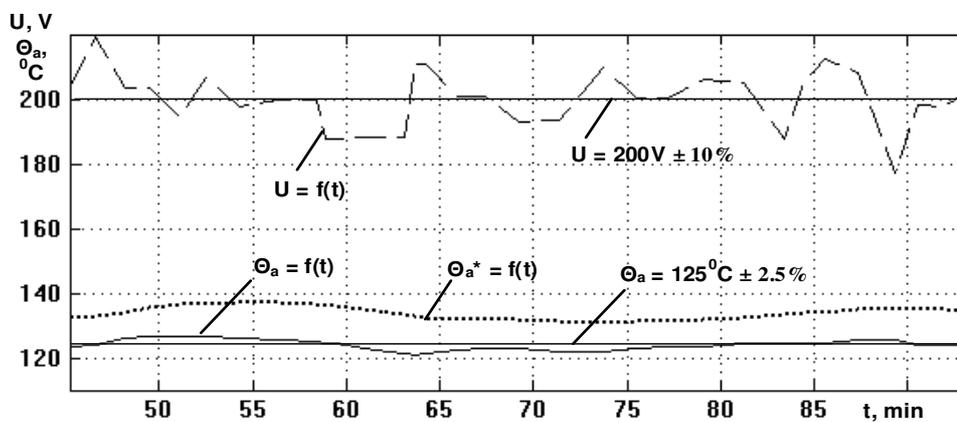
Fig. 8. Simulated characteristics of air mass temperature for stationary model ( $\Theta_a^* = f(t)$ ) and for non-stationary self-tuning up model ( $\Theta_a = f(t)$ ) under random variable voltage ( $U = 200 \text{ V} \pm 10\%$ )
