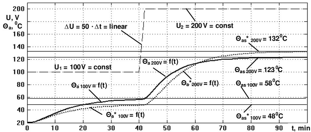
Fig. 5. Simulated characteristics of air mass temperature for stationary model ( $\Theta_a^* = f(t)$ ) and for non-stationary self-tuning up model ( $\Theta_a = f(t)$ ) under step and linear growing voltage ( $U_1 = 100 \text{ V}$ ,  $\Delta U = 50 \cdot \Delta t$ ,  $U_2 = 200 \text{ V}$ )
