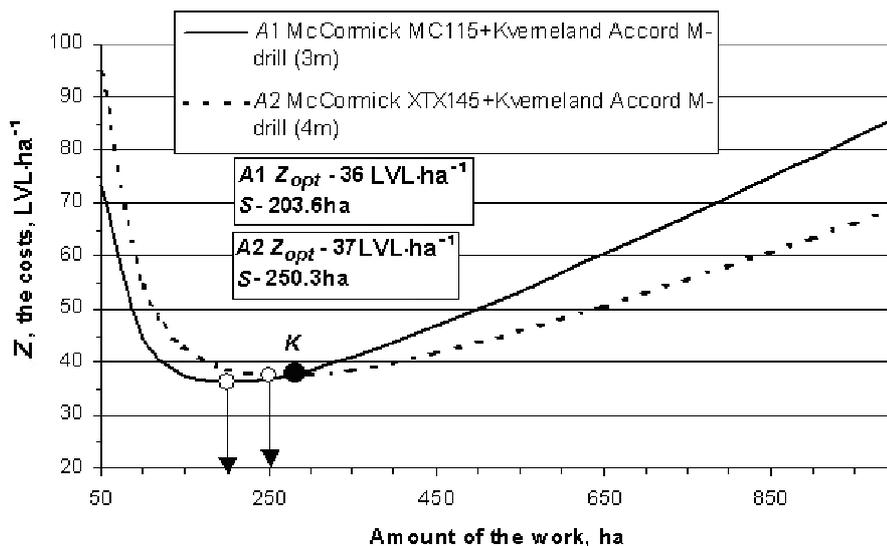
Fig. 3. Variations in the specific installed costs of the sowing aggregates depending on the amount of the performed work and the possible losses of the yields
