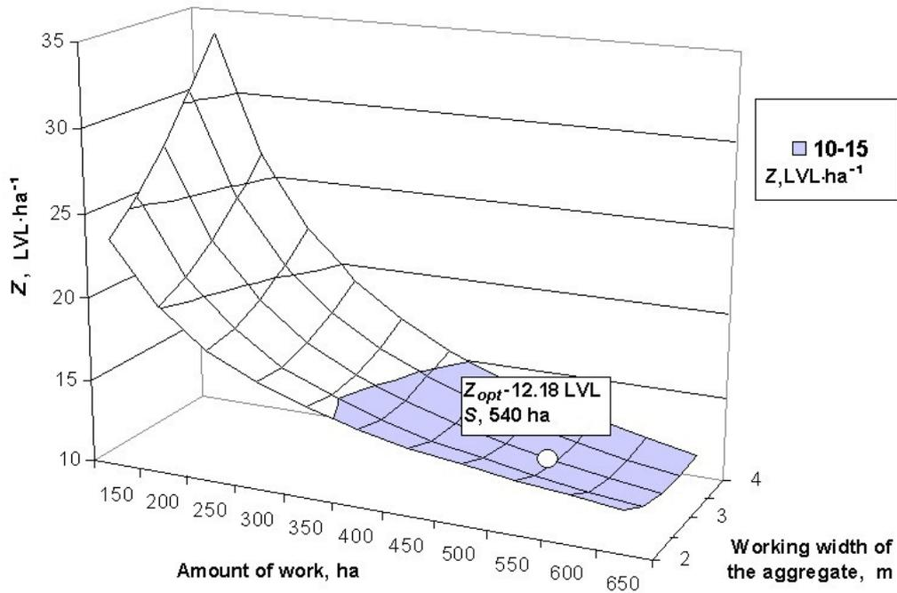
Fig. 1. Variations in the installed costs depending on the working width and the amount of work of the aggregate (aggregate McCormick MC115 + Kverneland Accord M-drill (3 m))
