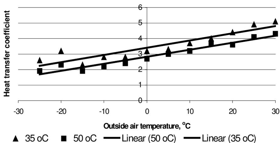
Fig. 1. Average energy transfer coefficient of outside air heat pump at the necessary temperature 35°C and 50°C (published data)
