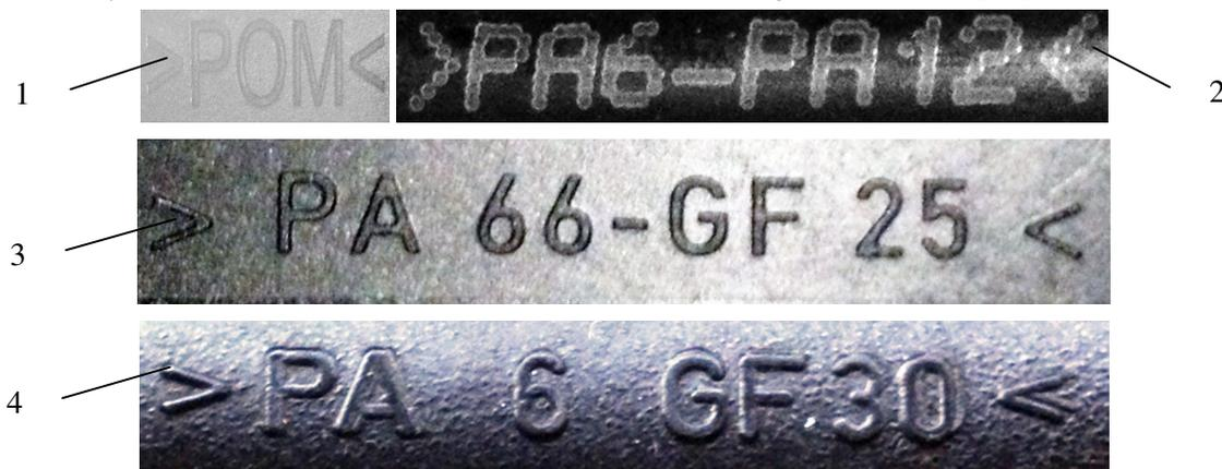
Fig. 1. Markings on polymeric parts: 1 – fuel pump container; 2 – fuel line; 3 – fuel vapor canister; 4 – fuel rail.
